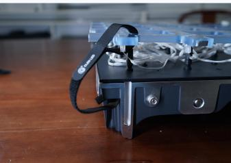
The string of lights is tied with a Velcro tape every meter, which is convenient for the string of lights to be stored, and the Velcro surface is relatively soft to reduce the damage of the string of lights
